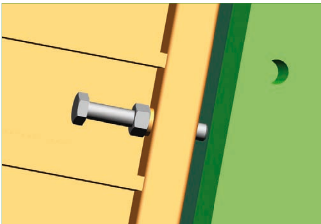
Fig. 2: Holding bolt pressing the WMC away from the frame; note the gap
